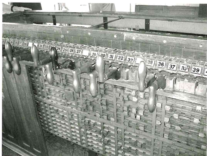
Electromechanical interlocking plant at the Southern Pacific RR tower in Santa Clara, Calif.
