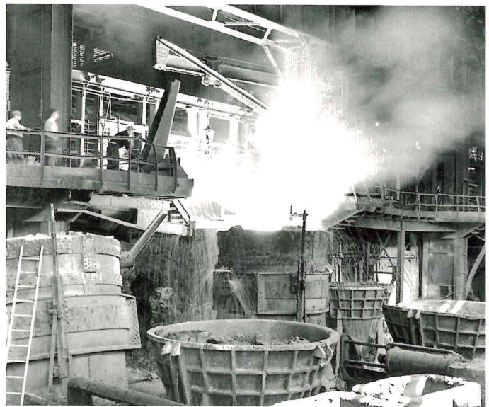
Otis Steel, ca. 1935. Tapping the open hearth.
