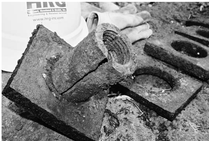
One of the cracked sleeves that contributed to the failure of the Kinzua Viaduct.
