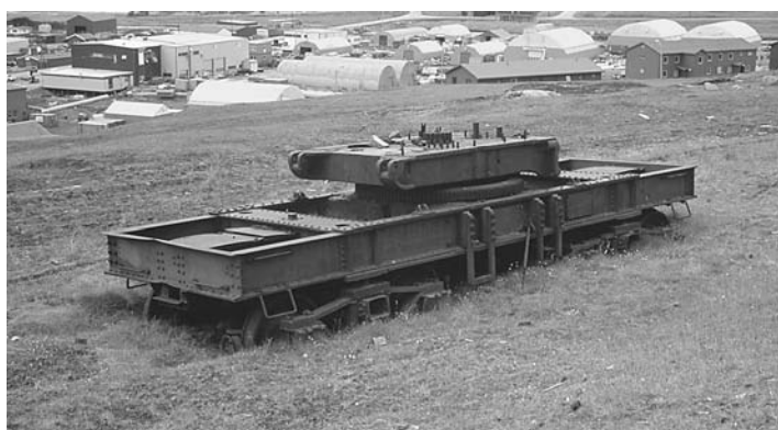
Substructure of Brownhoist crane with arch-bar trucks used by the Arctic Coal Co. to transfer coal between aerial tramway storage piles and rail tramway to the docks.
