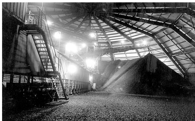
Inside the storage building at Hercules Cement, a system of conveyors continually deliver crushed limestone from the quarry. A slowly rotating radial bulkhead (left) delivers it to secondary crushers and mixers prior to processing in the rotary kilns.
