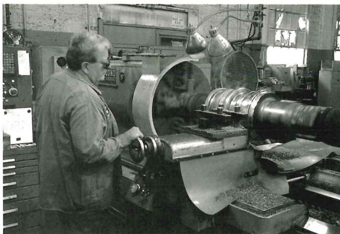
Machining a roll at McDonald Steel.
