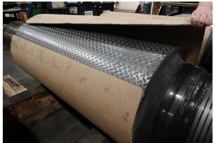
One roll from a pair of rolls used to press a texture onto sheets of metal at Rigidized Metals.
