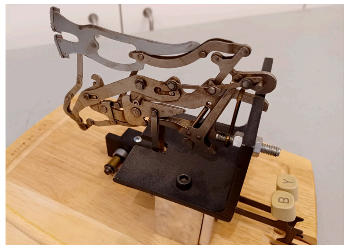
The elaborate mechanism for a noiseless typewriter key.
