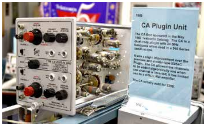
Model CA Plugin unit at Tektronix, introduced in 1959. Plugin accessory units were used to increase the scope’s versatility. Note vacuum tubes and other components of the era in well-organized cage-type construction. The red knobs in the voltage selector switches fine-tune the values.
