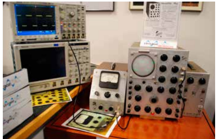
A square wave generator and first oscilloscope by Tektronix.
