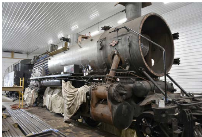
At the New York Susquehanna & Western Technical & Historical Society shop, front quarter view of Susquehanna 142, which is undergoing required inspection. The boiler, cylinder supply pipes, and cylinders have been stripped of their sheetmetal jackets and lagging (insulation) as needed for testing.
