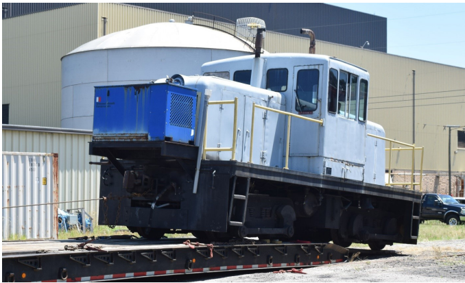
At the AdvanSix coal-powered power station, a trailer-mounted winch pulled the engine onto the specially rigged low boy where it will be secured for its ride to the ODC's Hallsboro yard.
