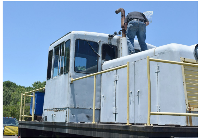
A final step before departure is the removal of the exhaust stacks to allow bridge clearance along the route.
