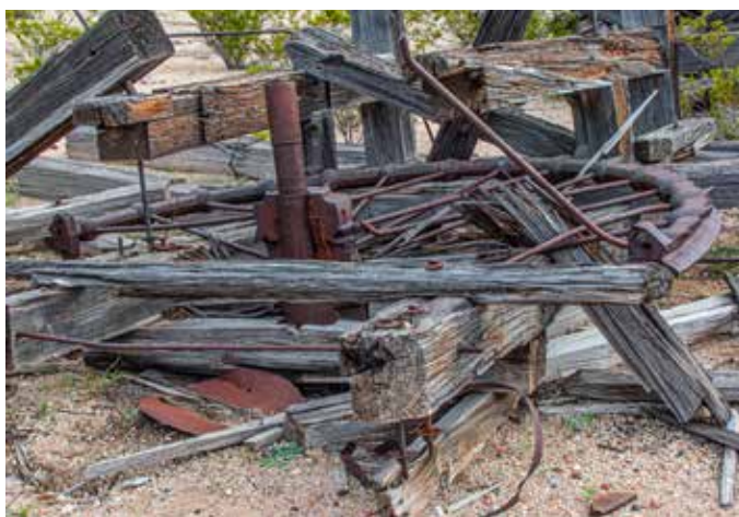
One half of the terminal's return wheel for the traction cable that moved the ore buckets. When compared to a historic image of the wheel published in Greenberg's article (2006), it appears one rim suffered accidental or deliberate damage.
