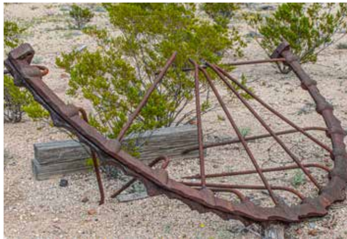
Presumably the other half of the ore terminal return wheel. Unlike the half wheel in the previous photo, strangely both rims are damaged. Noting the almost sprocket-like character of the rims, Todd Croteau and Dana Lockett, HAER architects involved in the Keane Wonder Mine tramway documentation, pointed out that the tramways need a ratchet system to ensure one-way traction cable travel, though it's not clear that's what explains the irregular rims.
