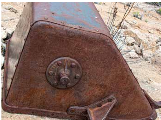
Buckets of unknown capacity like this carried ore from the mine in northern Mexico near Boquillas del Carmen. The bracket on the side (lower right) kept the bucket from tipping backward. A separate mechanism on the framework (missing), which hung buckets from the tramway, locked them from tipping forward until arrival at the ore terminal.
