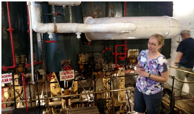
Viewing the Meteor 's original triple expansion engine, 1,195 HP, running at 75 RPM, powerful enough to tow one or two consort barges, doubling the 5,200-ton hauling capacity as a bulk freighter.
