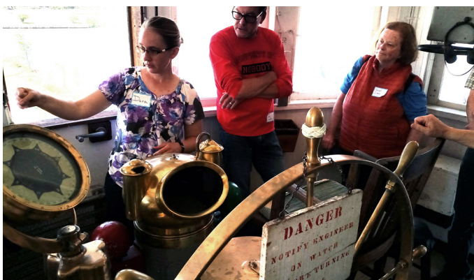
Dara Fillmore explains the chadburn (engine order telegraph), compasses, and other machinery in the pilothouse, which date from the original 1896 installation to additions in the late 1940s.
