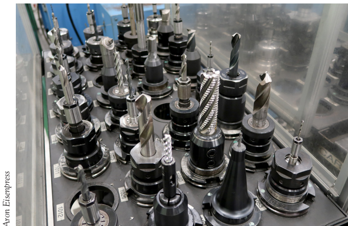
Drill bits at S&C Electric Co. used in an automated drilling machine.
