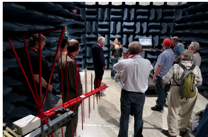
Anechoic chamber at Life Fitness, used for sound-level testing and for measuring electromagnetic emissions and radiation.
