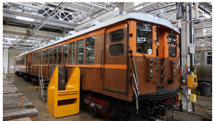
Skokie Shops, museum "L" cars 4271 and 4272, built in 1923. The Illinois Railway Museum (a stop on tour T2), has several sister cars. The marker lights under the front windows are used to indicate the train's route (this is still done on current equipment). These cars are part of the CTA Heritage Fleet and are fully operational.
