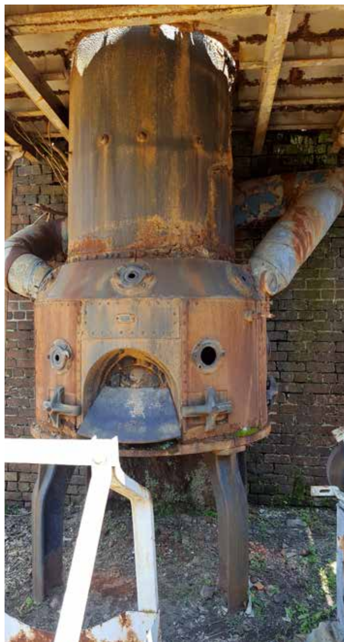
Cupola furnace at the Appomattox Iron Works.
