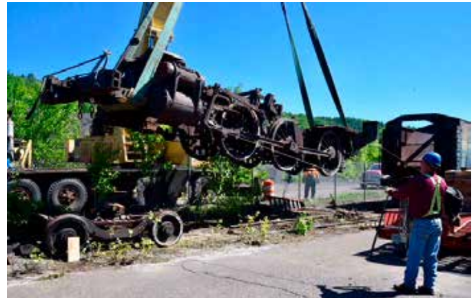
Lifting the locomotive frame and running gear.
