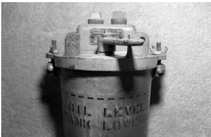
A small, never-used General Electric Co. oil switch. Height, 8 inches. Even more uncommon than a capacitor.
