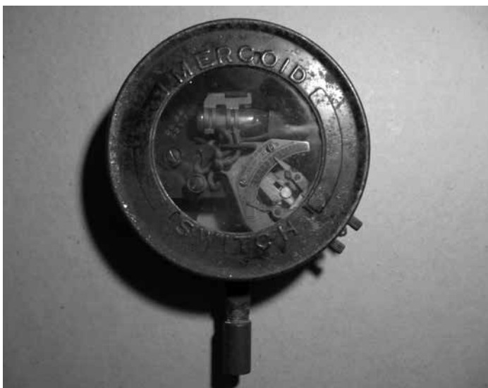
Intact Mercoild switch, patented Sept. 7, 1926. The mercury-containing glass vessel is visible behind the window. Diameter 5.8 in. The Mercoild Corp., Chicago, Ill.
