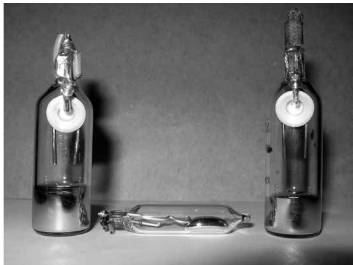
Mercury vessels removed from two Mercoïd switches. Height, 2 inches. For comparison, the small mercury switch is for residential use.
