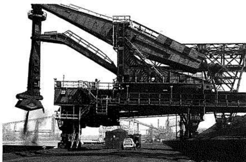
The Hulett unloaders at LTV's South Chicago Works The Hulett's bucket digs coal out of the barge's hold and drops it into a hopper in its framework for transfer to on-site storage. In the late 1890s, the Hulett's greatly improved the efficiency of ore handling, taking over for what was still largely a process of manual unloading.
