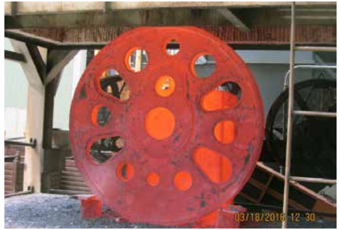
The T1's boxpok driver during the air-cool phase of the heat-treating cycle. The entire heat-treating process takes about two days with peak temperatures around 1,300°F.
