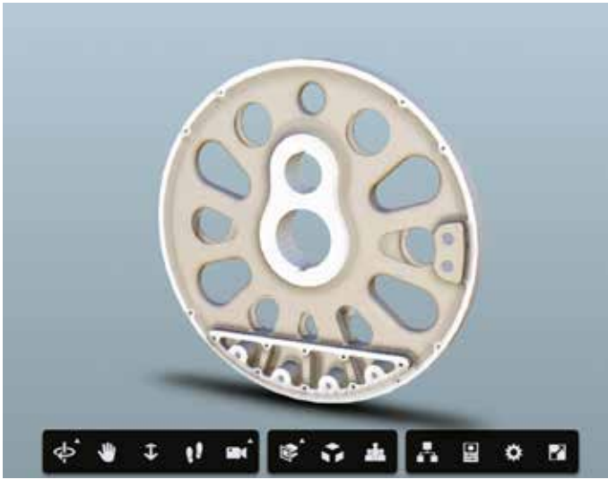
3D Rendering of the locomotive boxpok driving wheel.
