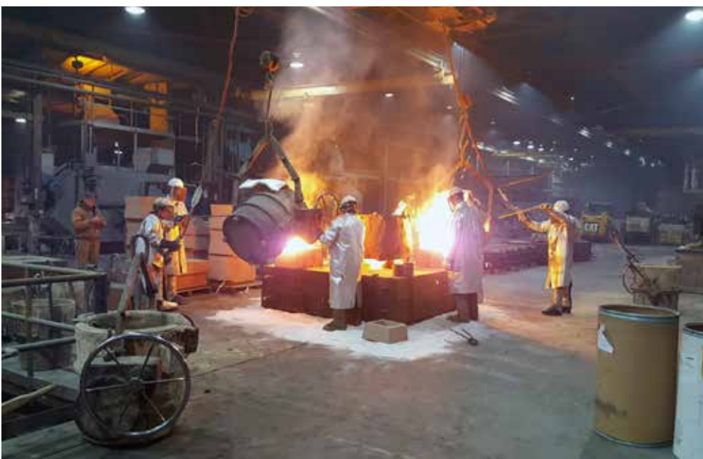
Casting the boxpok driver at Beaver Valley Alloy Foundry.
