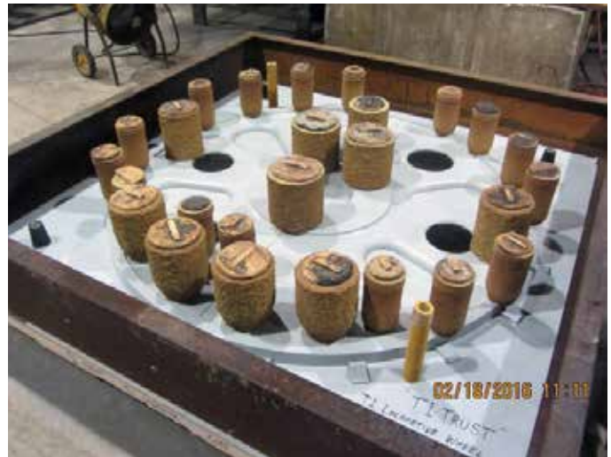
The boxpok driver mold, showing the cope half of the driver pattern with risers, aka feeders. The risers feed molten metal back into the casting as the steel cools and contracts. The use of the risers helps to prevent defects from forming in the casting.
