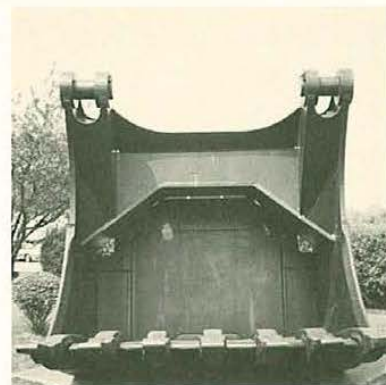
Among the smallest of the Marion Power Shovel Co.'s big buckets, this 20-cu. yd. dragline "dipper" is in a park at the plant site. Standing on its teeth, Bill Ellenberger [ SIA ] reveals the massive scale of even this small example.
