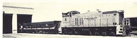
Right: At the end of the process at the Stickney Water Reclamation Plant, sludge ("dewatered wastewater solids") is conveyed [above] to a truck- and rail-loading facility. The Metropolitan Sanitary Dist. locomotive hauls sludge to drying areas in cylinder side-dump DIFCO gondolas [below]. R. Frame photos.
