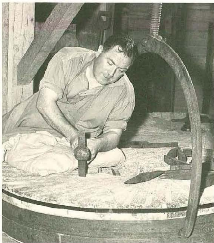
Charles Howell dresses a French-buhr millstone in 1971, Philipsburg Manor Mill. Courtesy Historic Hudson Valley.
