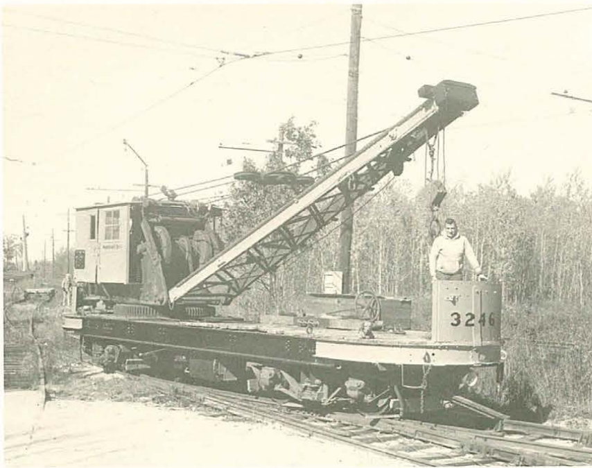
OF IA INTEREST AT THE SEASHORE TROLLEY MUSEUM. Left & above: No. 3246, trolley crane built by Industrial for Boston Elevated Rwy. in 1916. Left below: Wire-repair, roof-platform trolley no. 4, converted from a passenger car. Built for Claremont (N.H.) Rwy., date unknown. Since retiring to Seashore, it has been borrowed by Boston transit for occasional work duty. Below: Subway crane from Boston Elevated Rwy. Bottom: No. 2016, trolley flatcar built in 1912 for Boston Elevated Rwy. Photos courtesy Seashore Trolley Museum.
