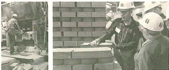
Pressing firebricks at the A.P. Green Refractory Plant in Bessemer, Ala.
