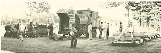
A brief stop was made at Brunswick to look over equipment once used for winter logging. Here, left to right, are a motor truck with caterpillar treads in place of rear wheels; a steam-powered Lombard Log Hauler, with treads and runners; and a pair of log sleds like those towed by the hauler.
