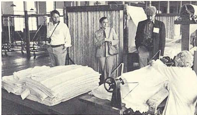
"Hooking" velvet at Cheney Bros. Prior to shipment layers must be separated by small hooks on the packing racks to avoid crushing the pile.
