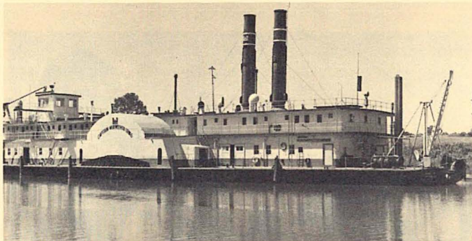
The Captain Meriwether Lewis , built by Marietta Mfg. Co., Point Pleasant, W. Va. 1931, first worked the Missouri River near Glasgow, Mo. 21 May 1932. Length — 269 ft.; 5 ft. width-85 ft. over paddle boxes; draft, loaded — 4½ ft. Sidewheels — 25 ft. diam. x 13½ ft.
