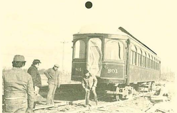
Moving the nearly restored Liberty Bell Limited into the shop on temporary trucks. Edward H. Blossom, restorer, at right. G. Wayne Laepple photograph.
