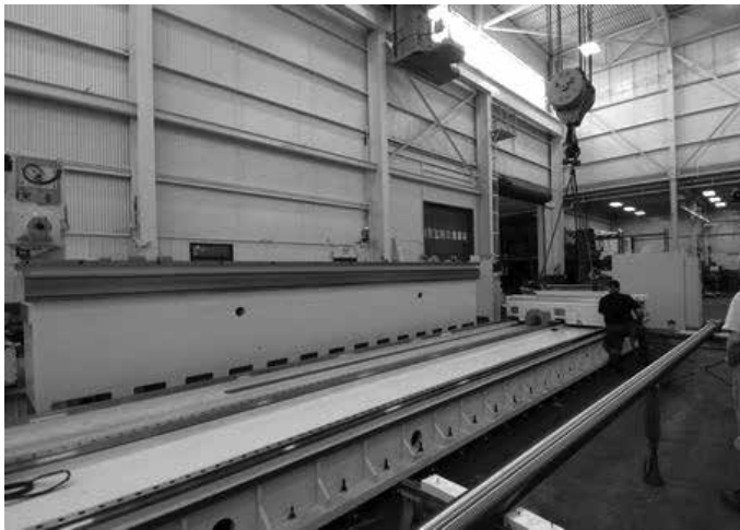
Boring mill for artillery gun tubes at Bourn & Koch.
