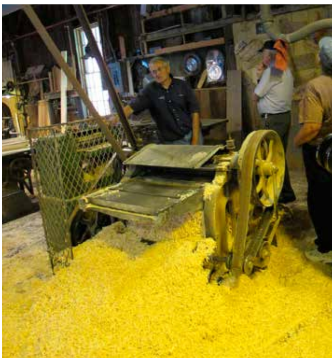
Alden Witham at Contractors Millwork sash shop explains operation of a Baxter planer.
