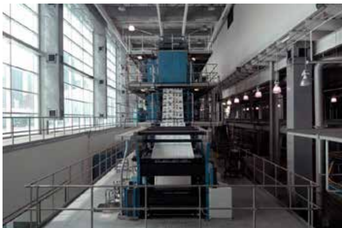
The German-manufactured Koenig & Bauer AG (KBA) web press at the Kansas City Star printing plant.
