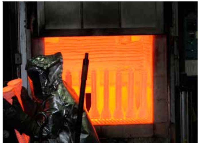
Worker at AMT removing a heated shell for casting.
