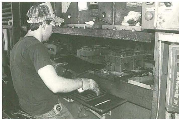
Taking shape. Baker Manufacturing Company makes furniture for the U.S. Postal Service. Particle board with a Melamine finish is produced in one section of the factory. In another, pressmen produce metal legs and drawers.
