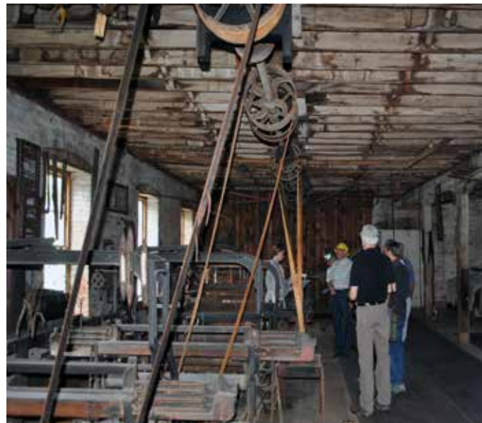
Looms and line-shafting inside the Watkins Woolen Mill.
