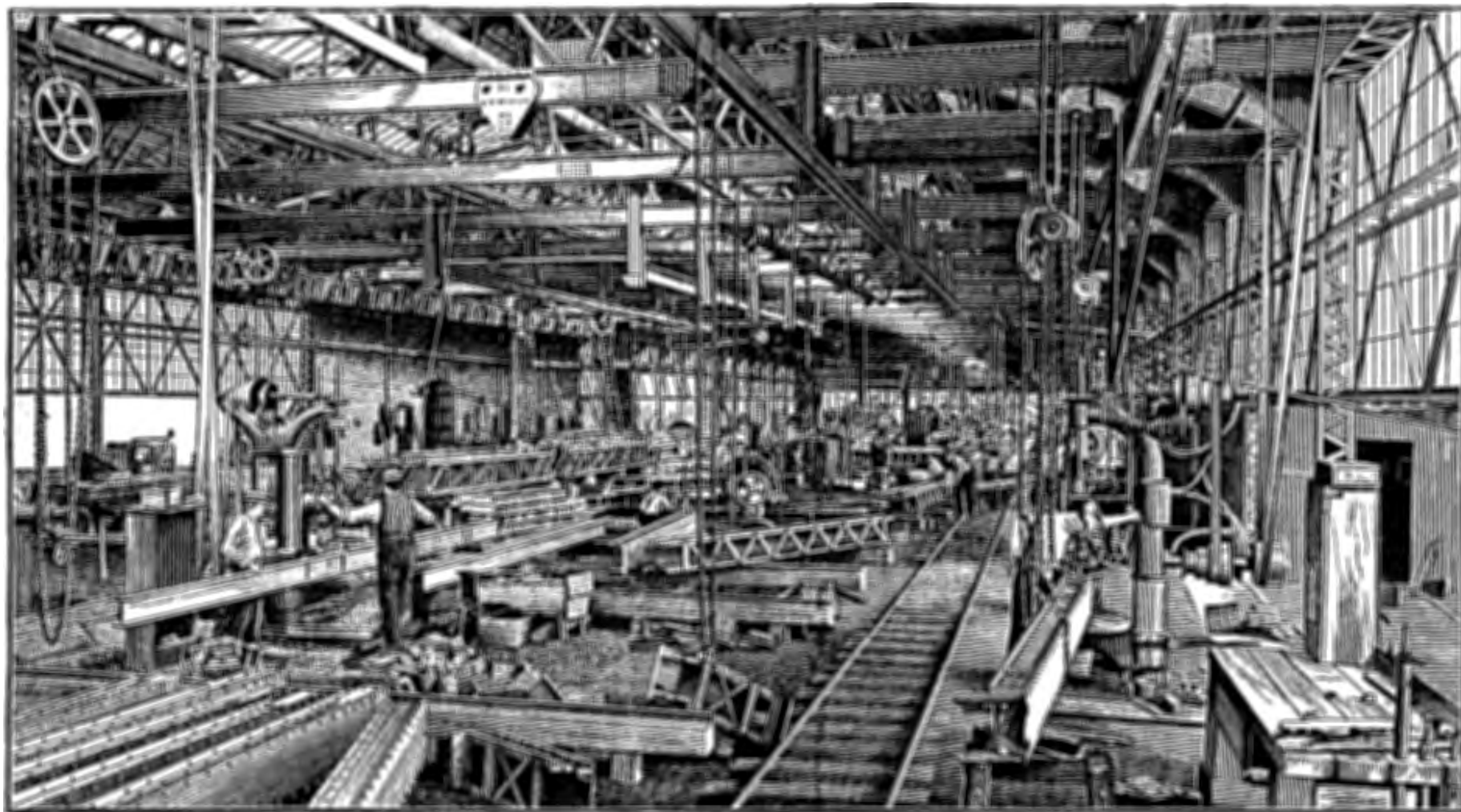
A well-appointed bridge shop of the 1890s. The 80-by-400-foot building—itsself presumably a product of the firm's works—was entirely of iron and glass with no wood used. The capacity was 1,000 tons of finished work per month. (Berlin Iron Bridge Company, East Berlin, Connecticut)
