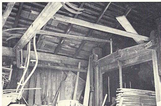
Saw frame and part of log-carriage feed mechanism. Donald Hutslar photograph. from a larger grouping that helped Ohio lead the nation in the production of corn whiskey in 1850.
