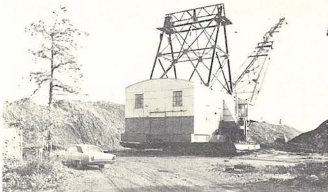
Walking dragline stripping shovel, near Eckley. The shovel is electrically powered, fed by cable from a remote source.
