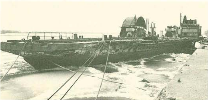
The Lansdowne on her knees—may she rise again. At right the wrecked engine. Seen is the piston, not the cylinder head which has left the scene. National Museum of Science & Technology photographs.
