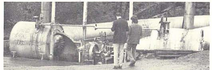
Pair of abandoned Leffel water turbines in "boiler-case" settings, with their governor, sans wheelhouse, at the U.S. Bunting Co. mill, Lowell. The vertical stacks absorbed surges in pressure caused by too-rapid closing of the control gates.
