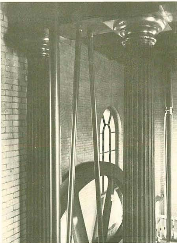
HAMILTON PUMPING STATION, 1858-59, designed by Thomas C. Keefer, C.E., compound steam pumping engines by John Gartshore, Dundas, Ont. Upper-left: main columns and one flywheel. Upper-right: high & low pressure cylinder heads, one set of crank-end valves, and watt-type parallel motion. Lower-left: pump and connecting-rod ends of the beams. Lower-right: the station and detached chimney. Ralph Greenhill photographs upper & lower left.
