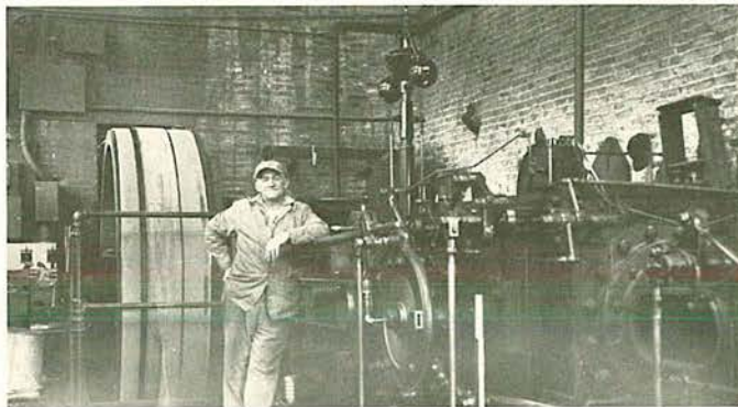
Pride of the Free State. Sauk Trail Line's C & G Cooper Corliss engine in its 2nd incarnation, at Acme Box Co, Baltimore (1954 photo).
