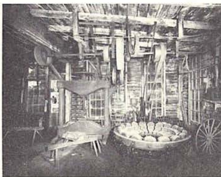
Gruber Wagon Works. (left) Exterior. (center) Blacksmith shop: hub press and hydraulic tire setter. (right) Wood shop: lathe and Gruber-built spoke-tennoning machine. HAER photographs by Wm E Barrett.
