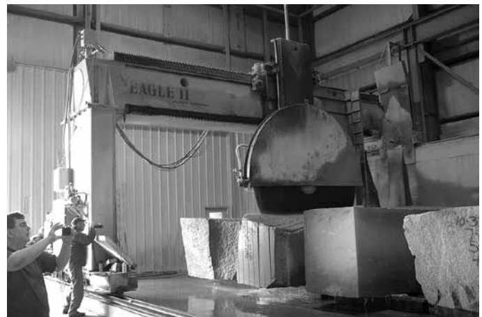
A giant circular saw cuts blocks of granite into slabs at Swenson Granite.
