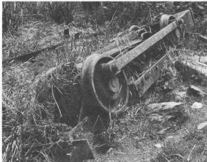
Beach Puzzle Picture. How many machine elements can you find ending their days on the beach near Juneau? Can you spot the lathe bed, the Pelton-wheel casing, the mine-car pedestal plate...? While on the right, scattered down a hillside below the Silver Queen Mine SE of Juneau is one truck of a Risdon Iron Works geared mine locomotive.
